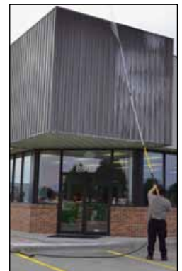
Telescoping wands extend to 24' to reach high places without scaffolding
